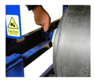
7. Insert the front locking pins to keep roll in place. One pin is required in each side frame.
