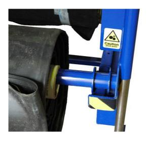
4. Locate the flanges on the lifting pole onto the carriage to keep in place.
